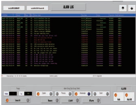
Screen displaying a list of all failures in the order of their occurrence.
